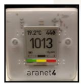
CO2 monitors work by giving an indication of how well-ventilated an area is, and therefore the potential concentration of a virus in the atmosphere.
